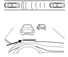
The vehicle will not stop unless the driver presses the brake pedal. If the brake pedal is pressed then braking is implemented with full brake function, even if the force on the brake pedal is light.
